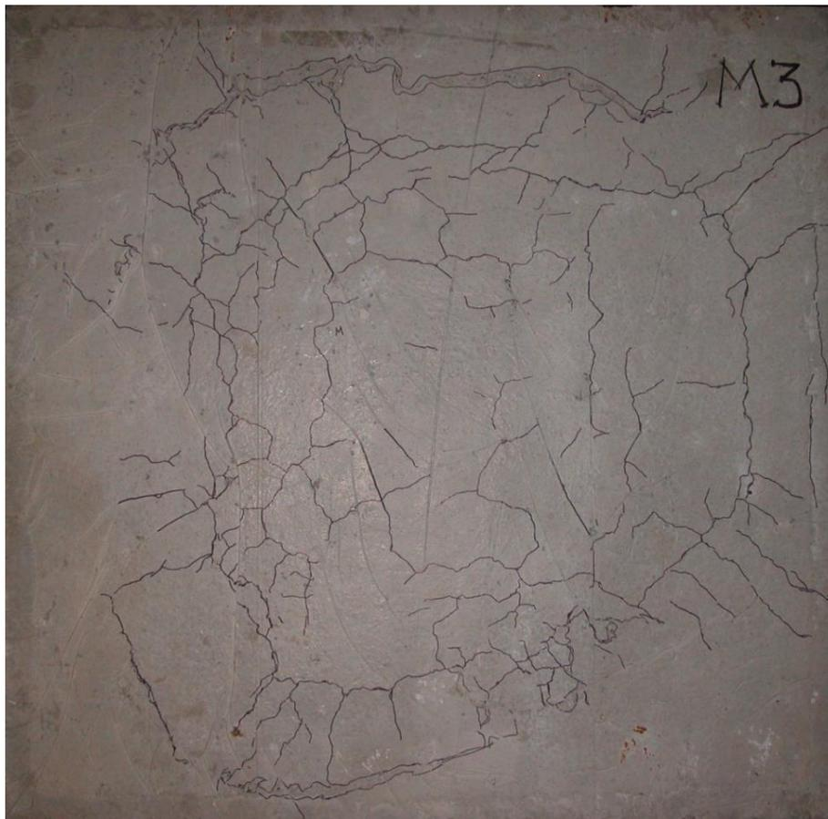
**Figure 3.** Lower (tension) slab face
