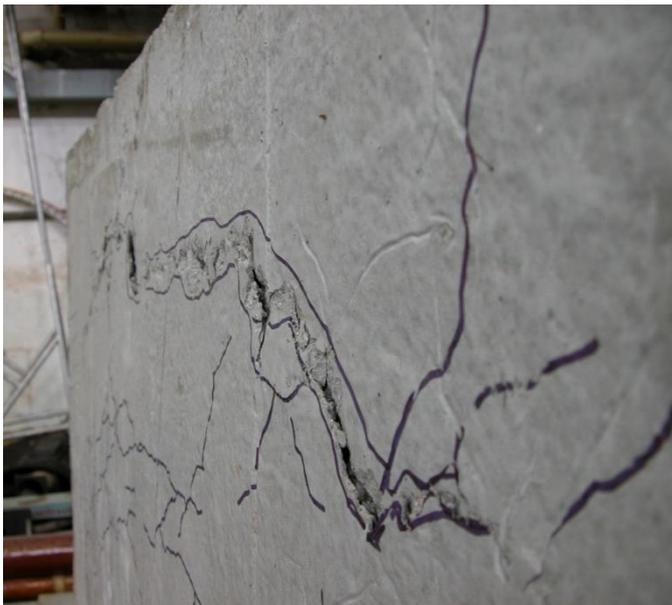
a) ring crack on the lower the slab face
